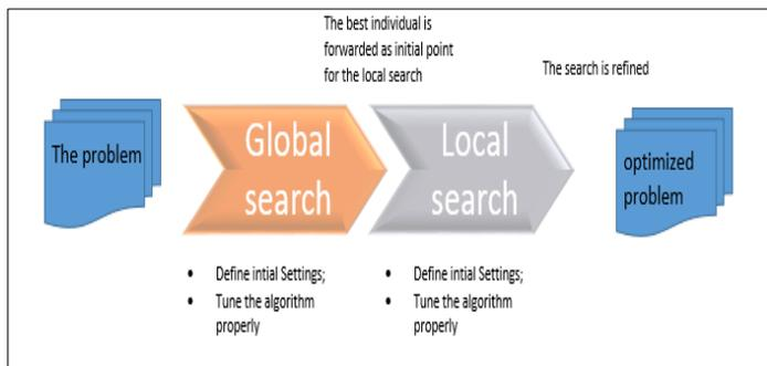
Figure 2: Schematic view of our hybrid algorithm. Source: Pires, 2017 [1]
