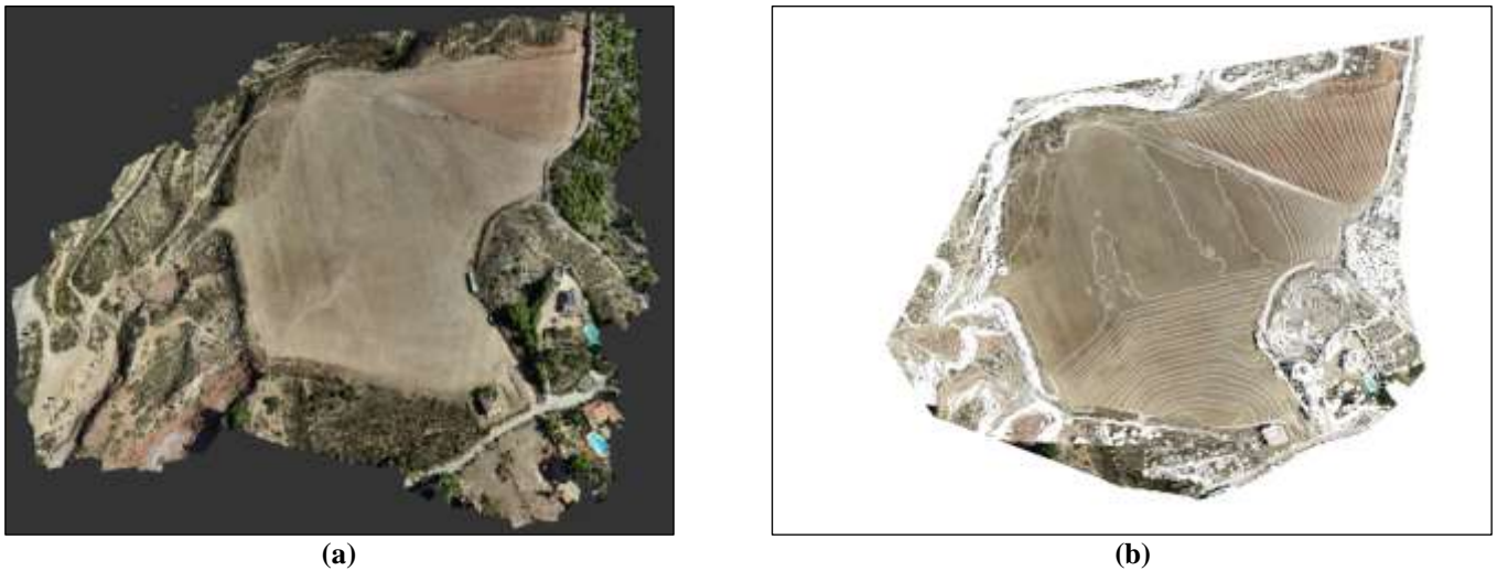
Figure 3: (a) LiDAR point cloud colored by Sitemark (b) Visual orthomosaic and contour lines based on the colored LiDAR point cloud.
