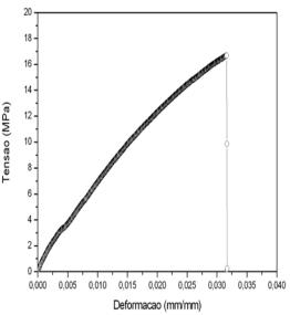
Figure 2. Typical behavior of the composite material based on polyester matrix and reinforced with 10mm length tauari fibers.
