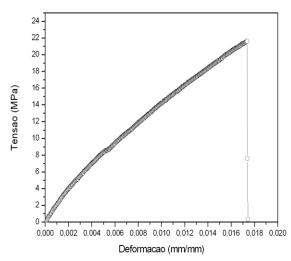
Figure 4. Force (N) versus extension (mm) of the composite materials reinforced with continuous and aligned tauari fibers.
