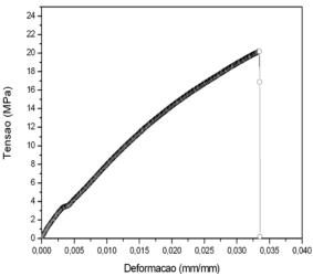
Figura 3. Force (N) versus extension (mm) of the composite materials reinforced with 15mm tauari fibers
