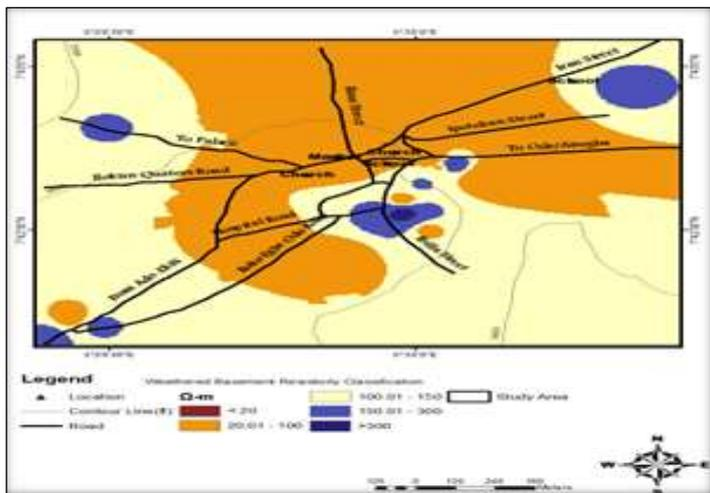
Figure 4: Classification of Weathered Basement Resistivity. Source: Authors, (2025).
