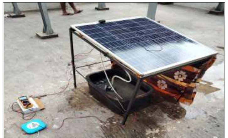
Figure 4: Wet Testing Setup with water Source: Authors, (2025).
